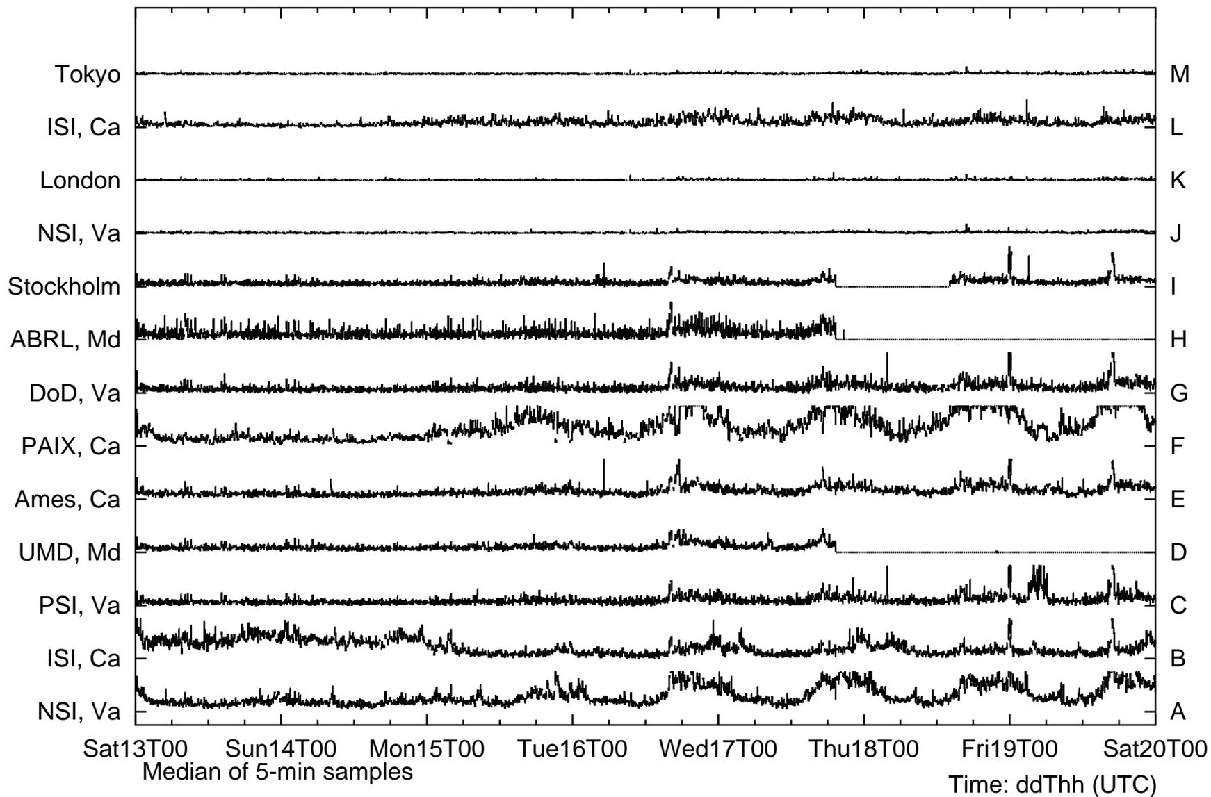
Fig. 1. Root requests per 5-minute interval, showing diurnal variation and loss of connectivity to D, H and I roots.
